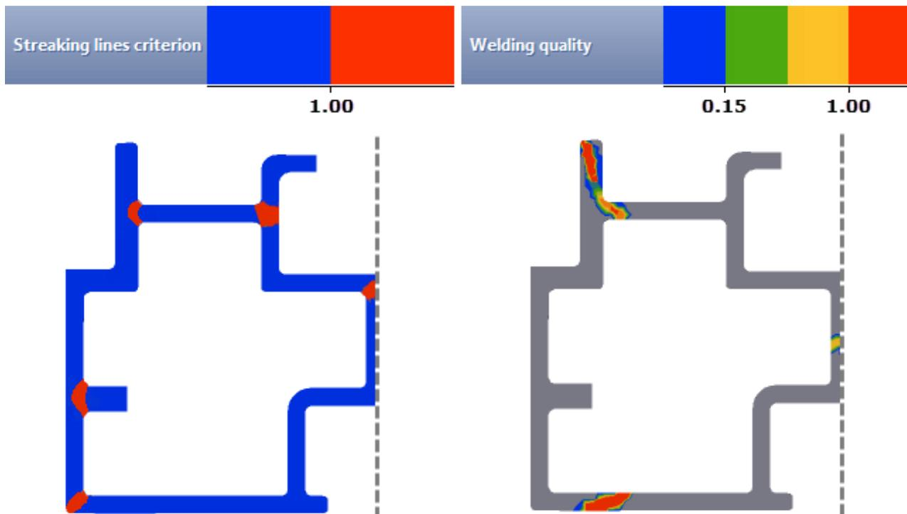
**Fig. 8.** Streaking lines (left) and welding quality (right) distributions calculated for the optimized design
