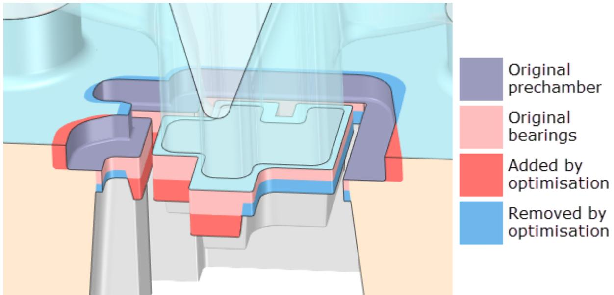
**Fig. 3.** On the explanation of optimisation procedure
