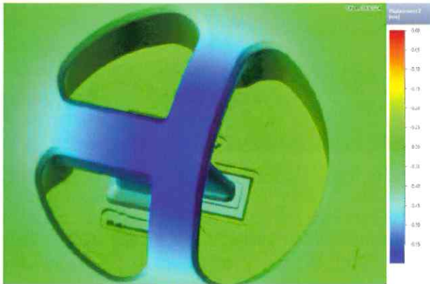
Figure 10. Axial displacement distribution in the third variant of the mandrel and web design.
