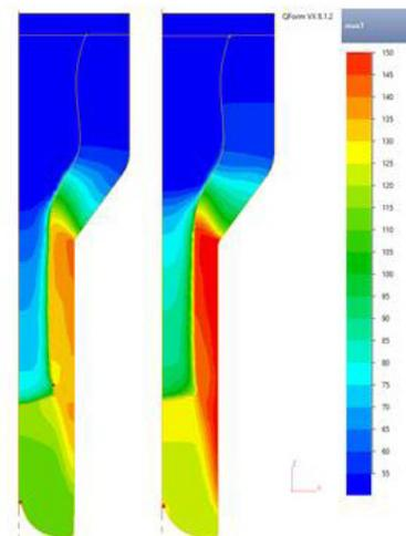
Fig. 8: Maximum temperature distribution in compacted PE. Extrusion of aluminum cup with inner diameter  $d=20$  mm and punch velocities  $v=50$  mm/s (left) and  $v=150$  mm/s (right) All simulation results are shown in table 1.
