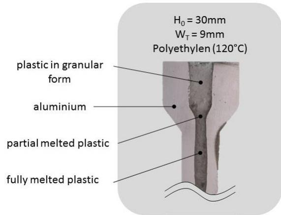
Fig. 5: Test part with three different melting sectors
