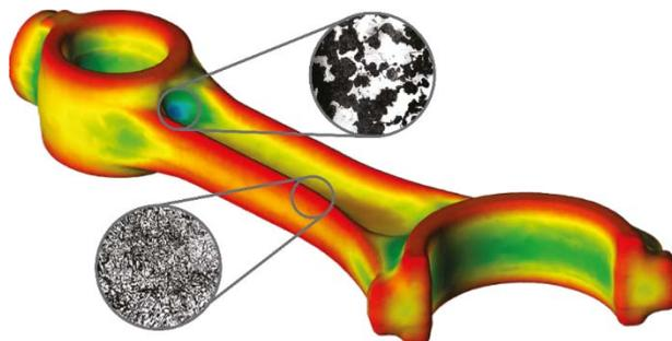
*Hardness distribution after connecting rod quenching. Bainite and Martensite phases are shown*
