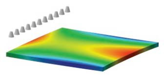
Thermo-elastic-plastic problem simulation. Distribution of vertical displacement shows distortion of the quenched steel sheet
