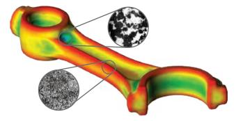
Hardness distribution after quenching. Bainite and martensite phases are shown
