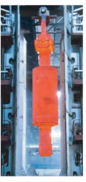
Quenching of the rotor in the sprayer device
